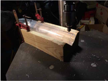
Photo 5: The jig used to ensure holes in the tubing were centered.
