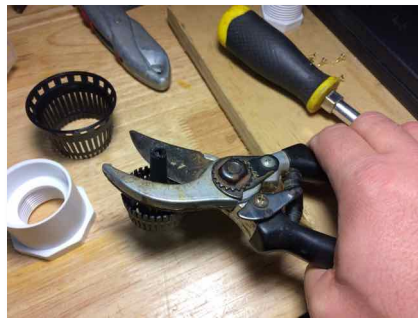
Photo 9: Trimming the center post off the strainer so it won't block the vent line.
