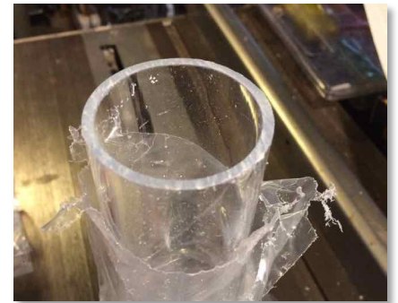
Photo 3: Acrylic tubing after being deburred.
