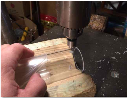
Photo 4: Drilling and countersinking holes for screws to hold in the end caps.
