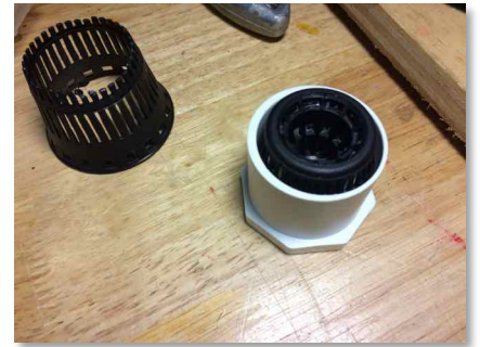
Photo 11: Drain screen installed in the end cap.
