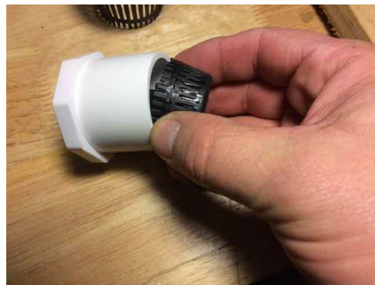
Photo 10: The strainer is simply friction-fit into the end cap. Silica gel beads will hold it in place.
