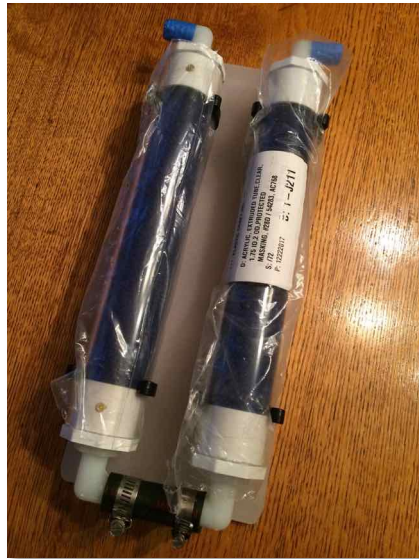
Photo 15: Finished assembly of the vent line dryer.
