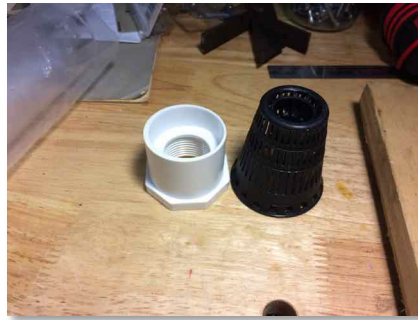
Photo 7: One end cap with a sink drain strainer that will be used to keep the silica gel beads contained.
