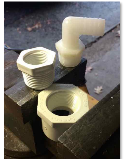
Photo 12: Parts making each end cap prior to being assembled.
