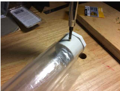
Photo 6: Driving in brass screws to hold the end caps in place.
