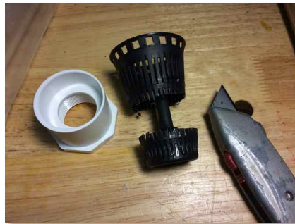
Photo 8: Sink drain strainer after it has been trimmed with a utility knife to fit in the end cap.
